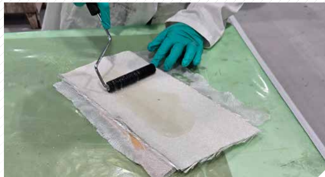
Rollers can be especially helpful at compacting multiple layers of reinforcing material, making for a stronger laminate.
