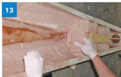
To fair the curves, 105/206/410 was spread as smoothly as possible with a plastic spreader.
