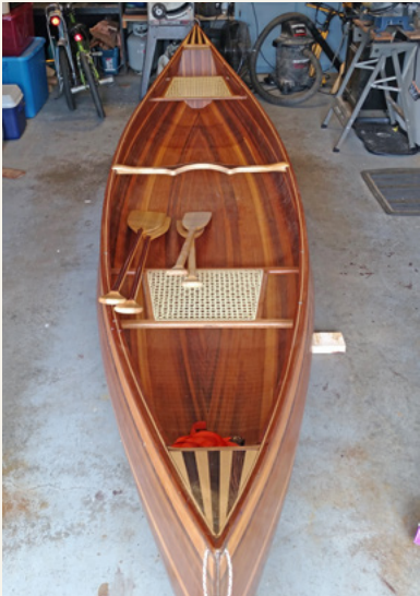
Jim Brown built this strip canoe in his New Hampshire garage. He used mostly cedar strips with some white pine and IPE on the gunnals. Using WEST SYSTEM® 105/207, he applied two layers of 6 oz. fiberglass to the bottom of his canoe and one layer to the inside.
