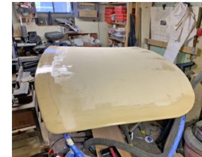
The hard top was sanded to remove all the high spots and start smoothing out the finish.
