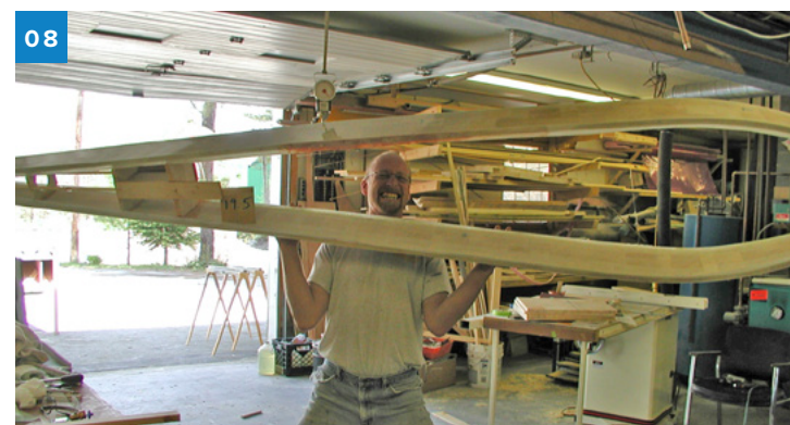
08 It was not necessary to fully assemble the fuselage on the strongback. Bonding the stem and stern blocks to the side panels while on the strongback made the fuselage dimensionally stable. This allowed the fuselage to be moved off the strongback and allowed the start of another set of panels. The stem blocks, mast step structure, and bulkheads only weighed 19.5 lbs.
