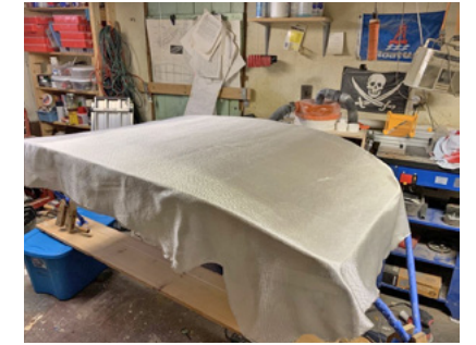
Two layers of 6 oz. fiberglass were applied to the foam core.
