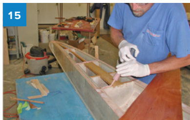
Epoxy thickened with 403 Microfiber was used to bond the epoxy coated okoume deck to the fuselage.
