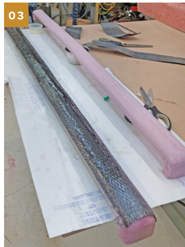
The foam was covered with carbon fiber to form the cross beams.
