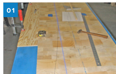
01 Cutting the 5/8" balsa core for the side panels of the fuselage.
