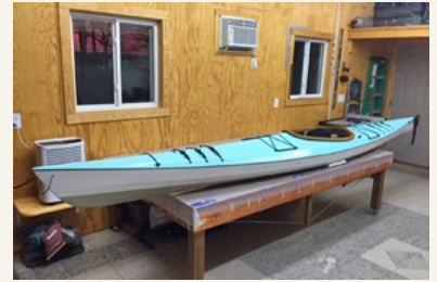
As a shipwright for 52 years, Mark Johnson has built many boats using WEST SYSTEM® Epoxy. One of which is this Pygmy Osprey standard kit kayak. He used stitch and glue construction. It is about 15 years old, and up until a year ago, it has lived it's whole life outside. Because of this exposure, he used AwlGrip® paint instead of varnish for UV protection. The bottom has WEST SYSTEM barrier coats followed by Bar Rust® epoxy, for a tough bottom. "She paddles like a dream, but tracks very straight, which is why I added the rudder."
