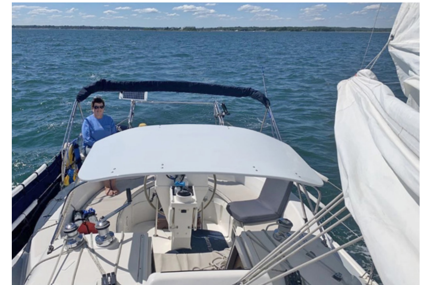
The finished hard top.
