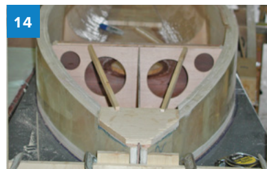
The seat back and bulkhead were epoxied in place.
