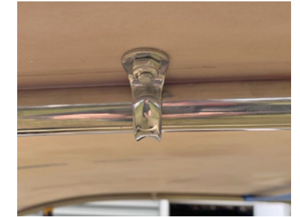
Stainless pad eyes with stainless steel bolts were used to mount the hard top.
