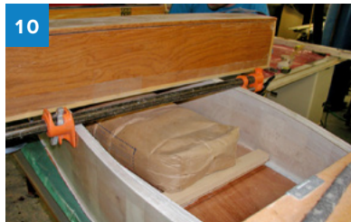
Okoume plywood was placed over top of the balsa core to finish off the cockpit floor. The fuselage side panels were weighed down with runner boxes, and sandbags were used to compress the cockpit floor laminate while the epoxy cured. Pipe clamps and a temporary spacer kept the sides plumb.
