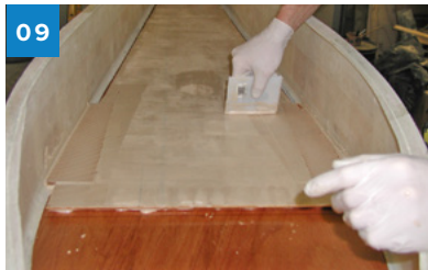
The bottom deck (1/8" okoume plywood) was coated with epoxy and placed on the strongback. Thickened 105/206 was applied to the angled fiberglass edge of the fuselage. The fuselage was bonded to the deck, followed by 5/8" balsa core reinforcing the cockpit area, and Baltic birch plywood in the plank attachment area. All layers were coated with thickened 105/206 on both sides using an 809 Notched Spreader.
