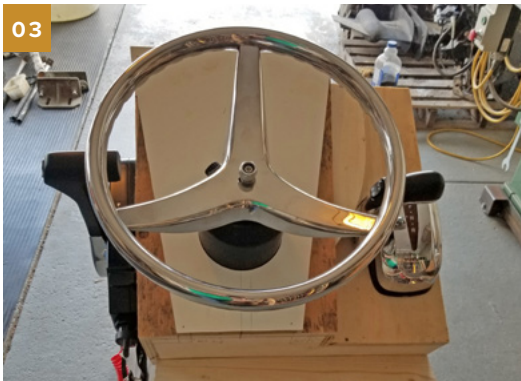
Rear station mock-up using scraps of plywood.
