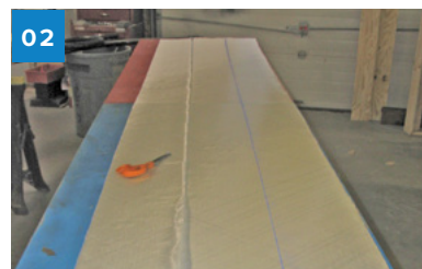
02 Cutting the +/-45 biaxial fiberglass fabric.
