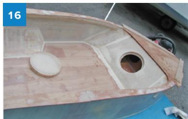
The rails are biased toward the inside of the cockpit, supported by the angled fiberglass edge of the side panels and the balsa core epoxyed underneath. This was shaped, and ultimately covered with 6 oz. fiberglass.
