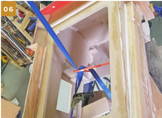
Prepping to laminate the second of the three mold parts.
