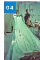
04 The layup of balsa, biaxial, and unidirectional fiberglass fabric was vacuumed to the mold. The blocks at the bow and stern were for exact length. 2x2 polystyrene foam on the side panel created angled fiberglass edges.
