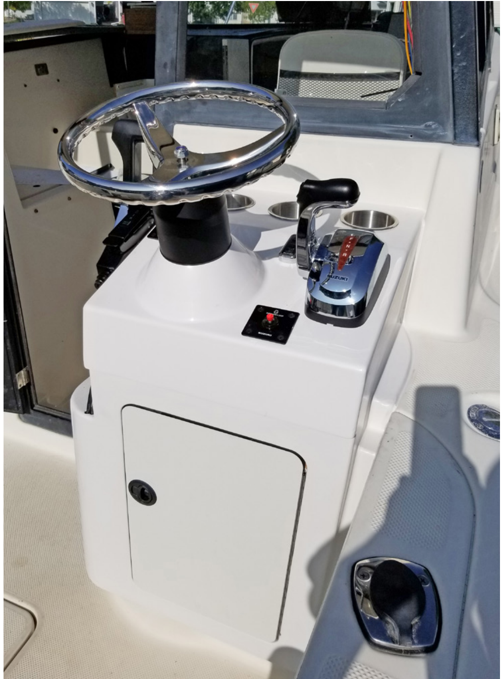
The completed rear station installed where the underutilized bait well used to be.
