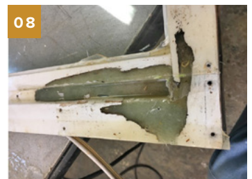
08 The epoxy cured and the mold was removed. Interior view.
