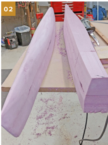
The foam was cut and shaped to form the hull.
