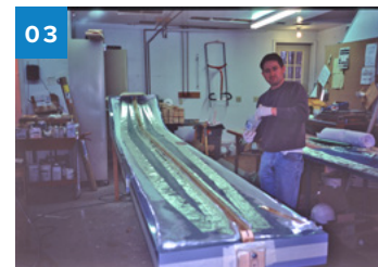
03 Unidirectional s-glass tape was used on the perimeter of the panels. +/-45 biaxial fiberglass was used on the inner and outer surface of the side panels. 6 oz. fiberglass fabric was used on the mold for a smooth, paintable surface.
