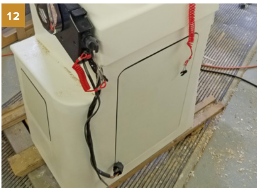
Fitting the doors for the battery switch and cabinet.
