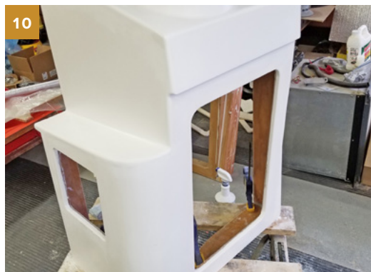
The rear station with all blemishes properly patched.
