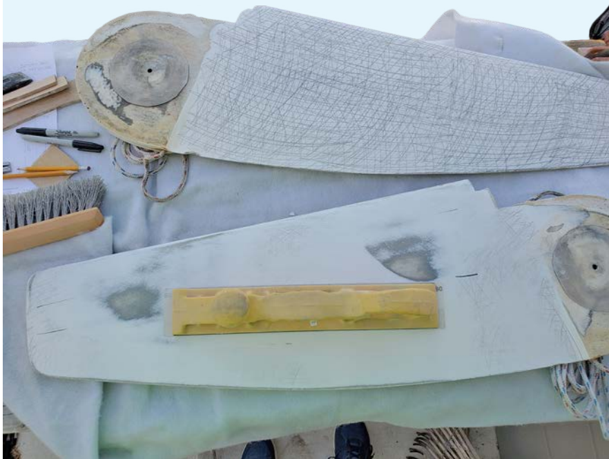
Most of the rudder has been shaded with a pencil, so after longboarding, you can see the fairness of the entire surface.
