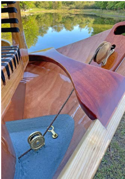
The rounded transom, mahogany transom brace, and custom designed aluminum block.
