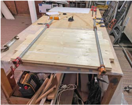
Tongue and groove pine was used for the base of the tub.
