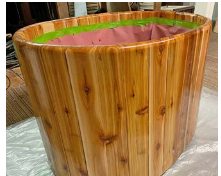
The entire tub was clear coated with 105/207.
