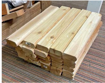
Cut 2x4 cedar strakes, with a bead and cove edge, formed the walls of the tub.
