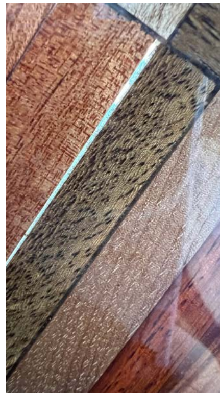
Small gaps between the wood samples filled with clear epoxy.
