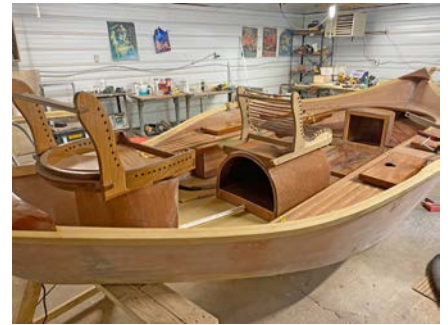
The boat after all major components had been completed. It's ready for the application of finishes.
