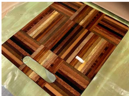
A flood coat of 105/207 was poured over the board for a high gloss finish.
