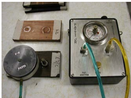
Pneumatic Adhesion Tensile Testing Instrument used to test the adhesion to wood samples.
