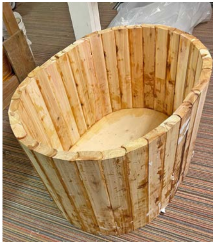
Once the epoxy cured, the tub needed to be sanded and the vertical strakes trimmed.
