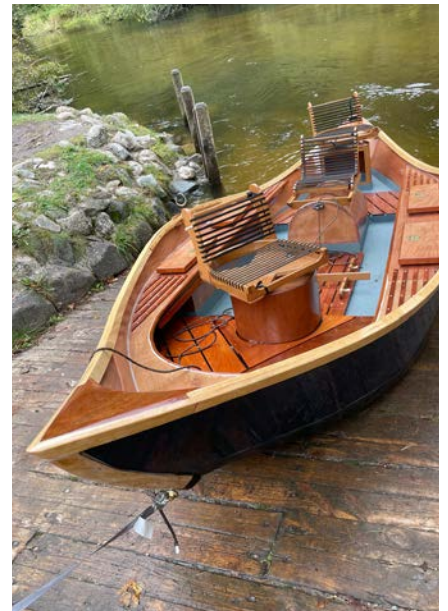
Front seat and pedestal, herringbone mahogany sole, and interior okoume deck with mahogany decorative trim.
