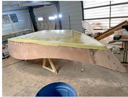
The boat after primary hull construction. Note the rounded transom on the right, recurve sides, and Kevlar fabric on the bottom and chines.
