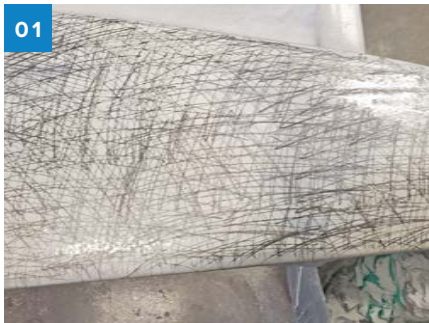
01 When marking the surface, you need to scribble in multiple directions so the low spots are obvious after sanding.
