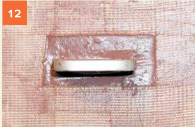
Surrounding hardware that penetrates the deck with epoxy, prevents moisture from reaching the core.
