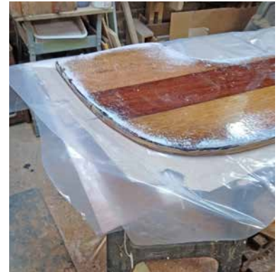
The veneering stack: the transom to be veneered, epoxy thickened with 403 Microfibers, veneer, plastic sheet, cardboard, plastic sheet, and the other transom. The cardboard helped to distribute the pressure.
