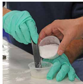
Thickening the epoxy with 404 High-Density Filler.
