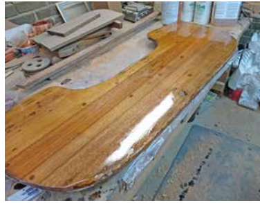
The original transom, glassed with 4 oz. and three coats of WEST SYSTEM 105 Resin ® /207 Special Clear Hardener ® .
