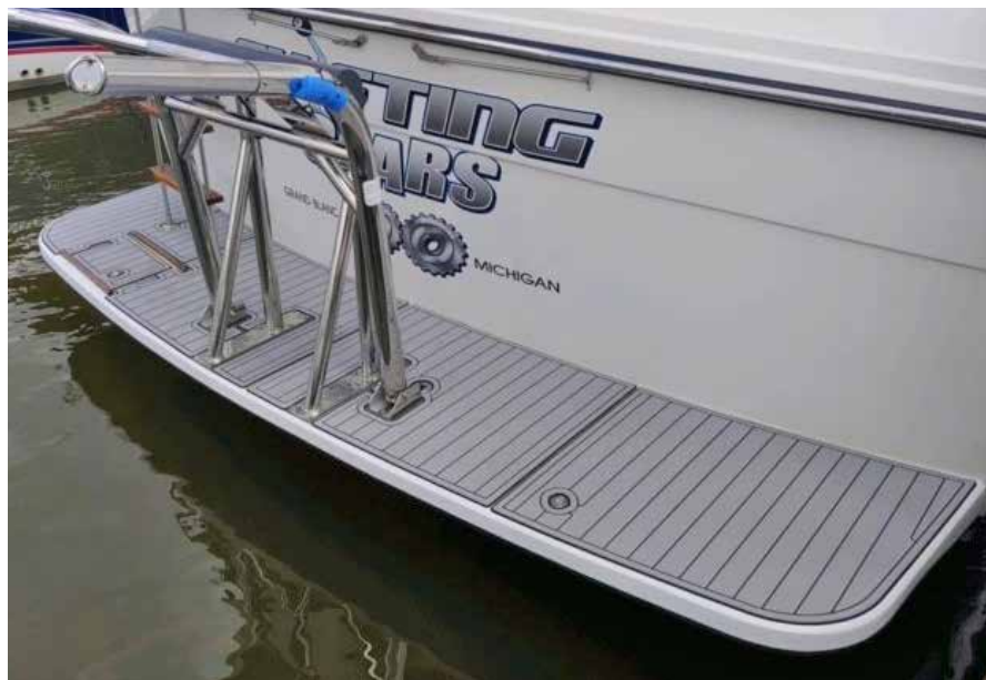
The finished swim platform newly reinforced with balsa core and plywood.
