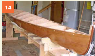
14 Hull upright - ready to plank deck.
