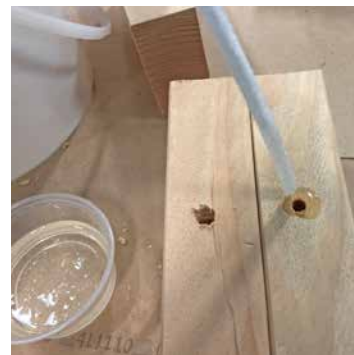
Wetting out the oversized hole.
