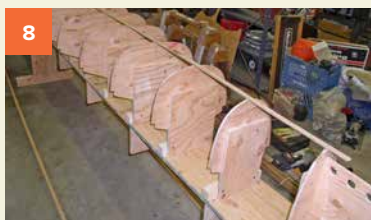
Batten mounted on station molds.
