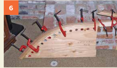
Bending stems on stem molds.
