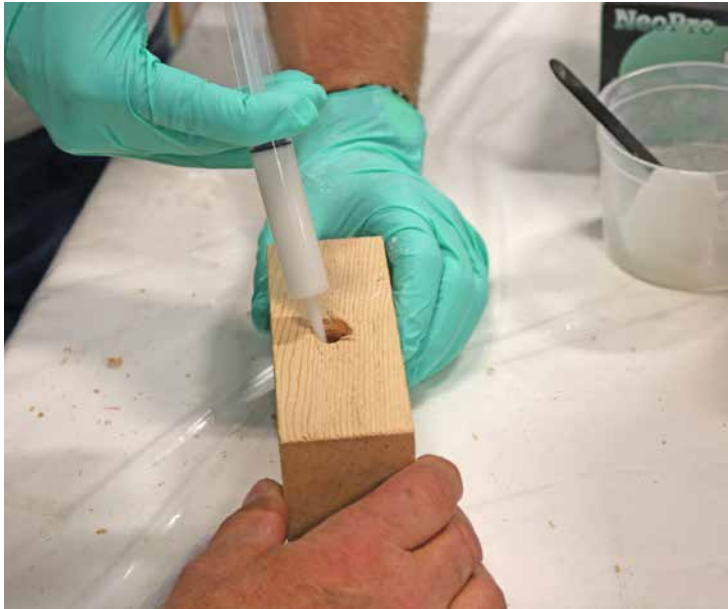
Filling the hole with the thickened epoxy.
