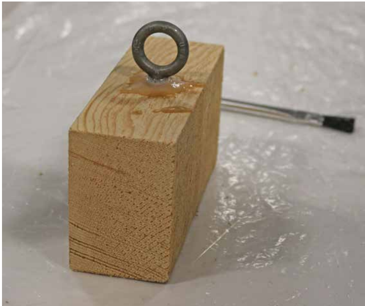
Added the fastener to the pilot hole.
