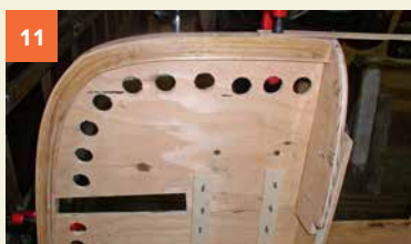
Internal stem mounted on stern stem mold.
