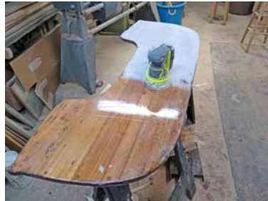
The 105/207 coating was sanded with 40-grit in preparation of applying the veneer.
