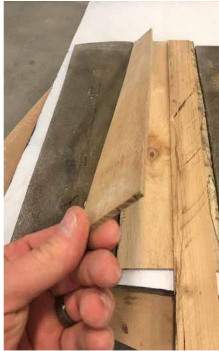
The pallet boards after being ripped down.
