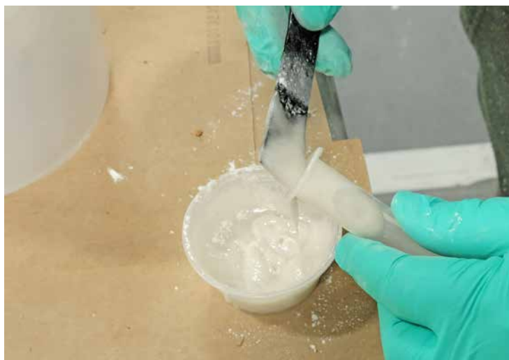
Filling the syringe with the thickened epoxy.
