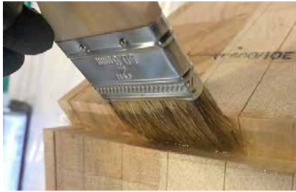
Coating balsa kerfs with epoxy.
