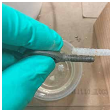
Wetting out the fastener.
