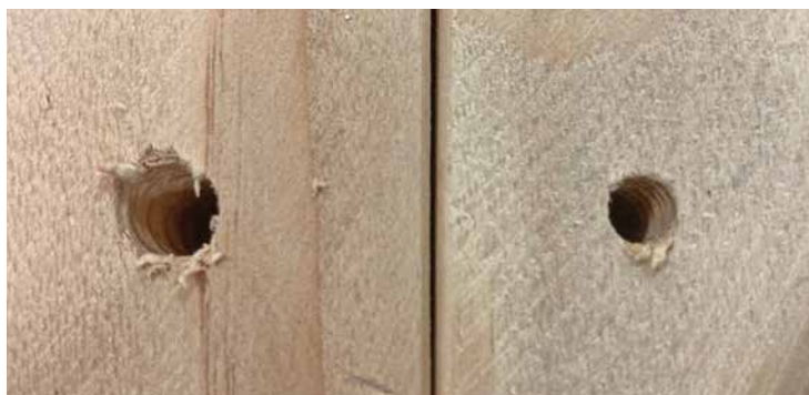
Oversized and standard pilot hole sizing.
