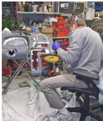
Applying a layer of 6oz. fiberglass with G/flex 650.
