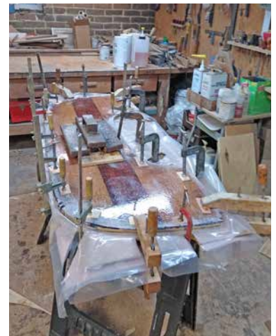
A heavy center weight and clamps around the edges completed the setup.
