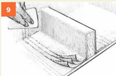
Staggering fiberglass tabbing layers minimizes concentrated stresses.
