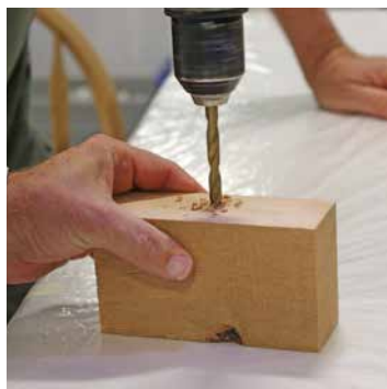
Drilling the oversized hole.
