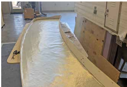
Fiberglass cut and dry fit.
