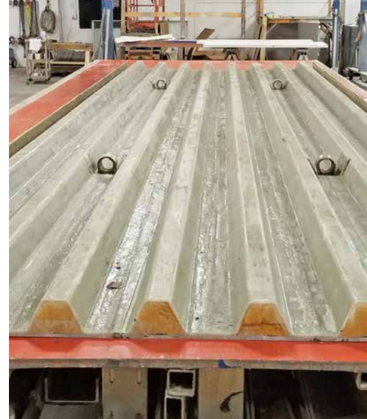
Close-up of the SC FRP bridge deck fabrication.
