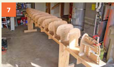
Stern mold mounted on strongback.
