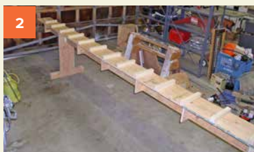
Strongback with mold stations attached.
