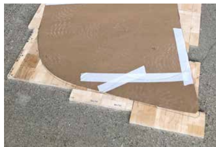
Using template to trace the new balsa core.
