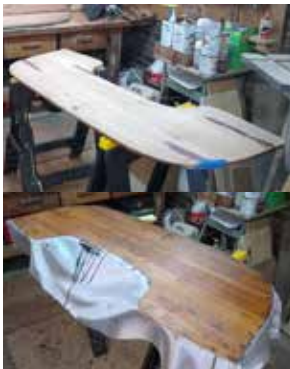
Repairing and glassing of the transom. The original transom was made up of two mahogany sections bolted onto the thin fiberglass hull's transom.
