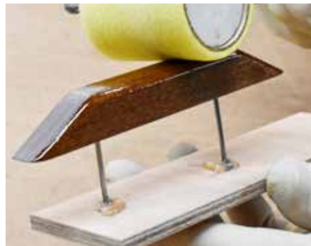
Left: The part is sanded between coats of 105/207 with a fine grit sandpaper for a smoother finish. Middle: The roller provides the most even film thickness. Supports need to be tall enough so all sides can be coated. Right: Once the epoxy is rolled on, it should be tipped with a foam brush for a smooth finish.
