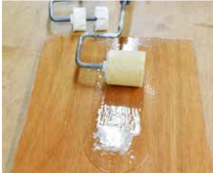
Left: To limit waste, use a scrap of plywood, and cut the roller down to the size you need. Middle: The support screws were hot glued on top of the plywood base giving maximum height for coating. Right: This small part was hot glued to a small support block.
