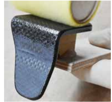
Left: To limit waste, use a scrap of plywood, and cut the roller down to the size you need. Middle: The support screws were hot glued on top of the plywood base giving maximum height for coating. Right: This small part was hot glued to a small support block.
