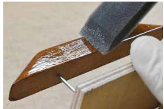
Left: The part is sanded between coats of 105/207 with a fine grit sandpaper for a smoother finish. Middle: The roller provides the most even film thickness. Supports need to be tall enough so all sides can be coated. Right: Once the epoxy is rolled on, it should be tipped with a foam brush for a smooth finish.
