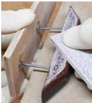
Left: The part is sanded between coats of 105/207 with a fine grit sandpaper for a smoother finish. Middle: The roller provides the most even film thickness. Supports need to be tall enough so all sides can be coated. Right: Once the epoxy is rolled on, it should be tipped with a foam brush for a smooth finish.
