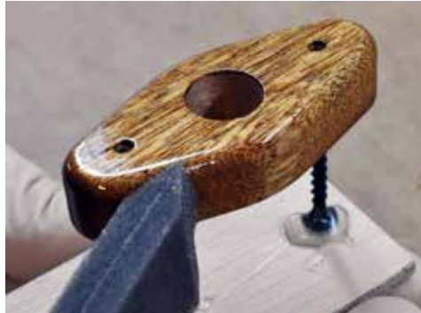
Left: To limit waste, use a scrap of plywood, and cut the roller down to the size you need. Middle: The support screws were hot glued on top of the plywood base giving maximum height for coating. Right: This small part was hot glued to a small support block.
