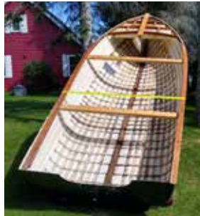
The inside of the boat cleaned, sanded, and ready for paint.
