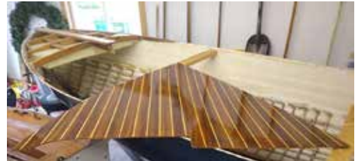
The new teak and holly foredeck with three coats of WEST SYSTEM 105 Resin/207 Special Clear Hardener® and seven coats of Captain's Varnish 1015.
