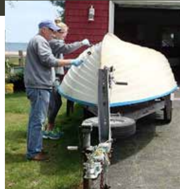
Applying three coats of WEST SYSTEM® 105 Epoxy Resin®/205 Fast Hardener.
