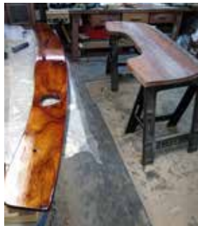
The cockpit dashboard with three coats of WEST SYSTEM 105/207 and seven coats of varnish.
