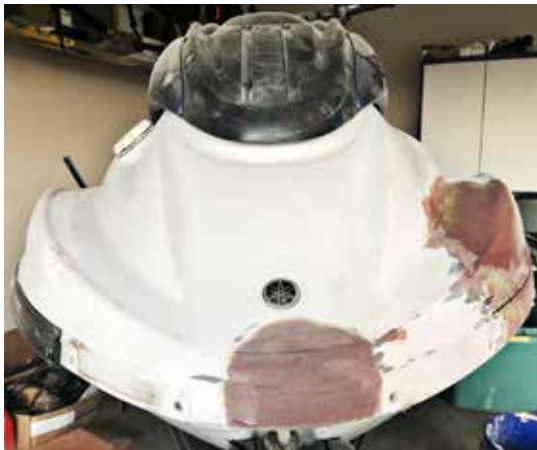
Besides the large crack on the side of the nose, there was a smaller crack on the front of the nose. The smaller repair was used for practice before attempting the larger repair.
