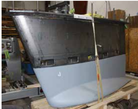
The 60-gallon fuel tank mounted on top of the bulb keel.
