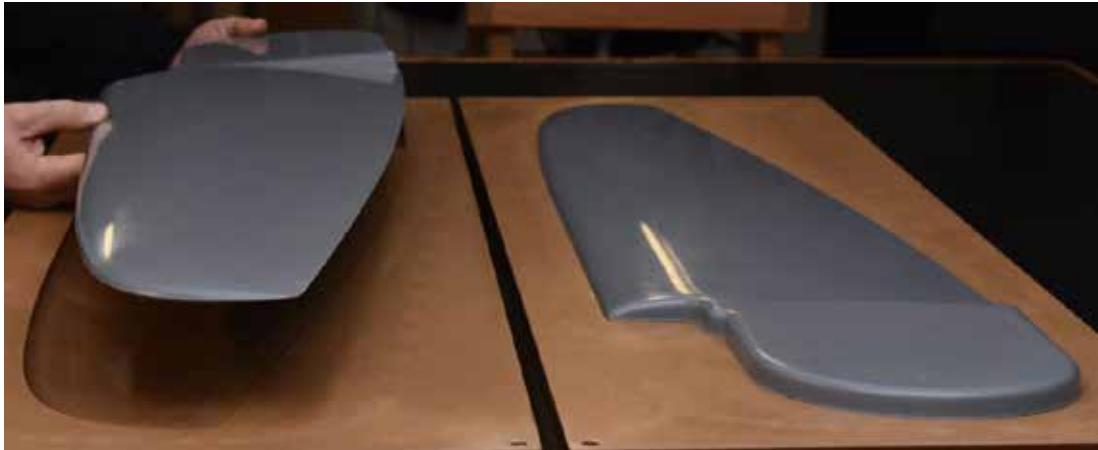
New rudders were built in two halves in CNC machined female molds. They were constructed using many layers of carbon fiber for the skins and a foam core with a large wooden shear web in the fattest part of the foil. They are a bit more modern (higher aspect) than the stock rudders and just over half the weight of the originals.
