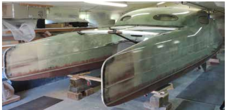
Above: The G-32 gelcoat has been chipped off, the low areas filled and then faired with long boards. The whole boat was coated with 105/207.
