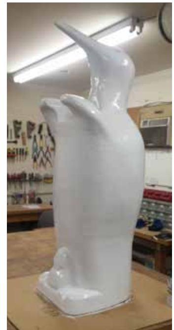
The first "primer" coat applied to the faired surface.
