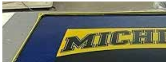
Vacuum Bag Sealant was a simple way to create a perimeter wall for a shallow pour.
