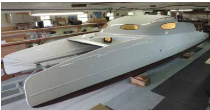
Above: The G-32 gelcoat has been chipped off, the low areas filled and then faired with long boards. The whole boat was coated with 105/207.
