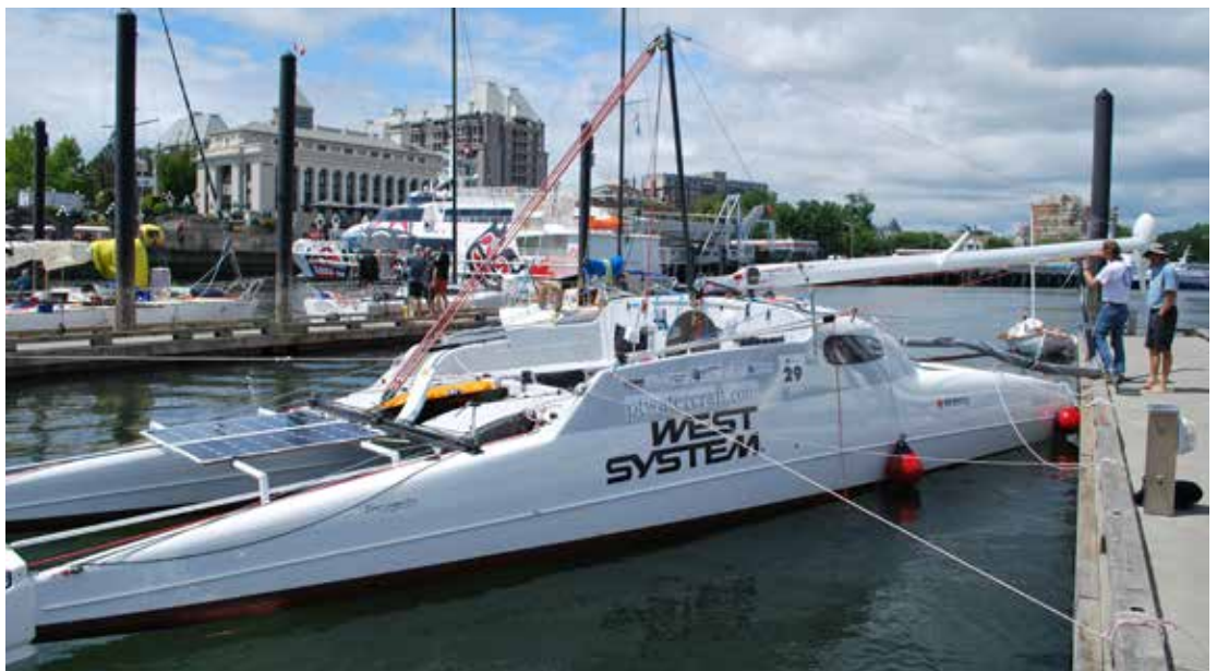
The boom is used as a jin pole to raise and lower the mast.
