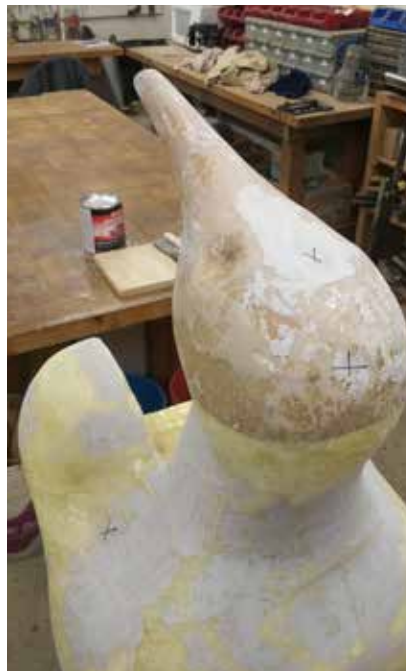
Bondo was applied to fill slight dimples after fiberglassing.
