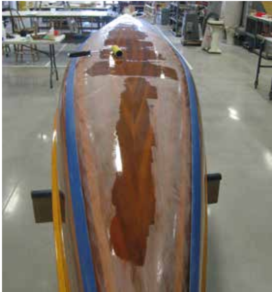
Localized coats were applied only to the low spots on the bottom of the canoe to build up the thickness.
