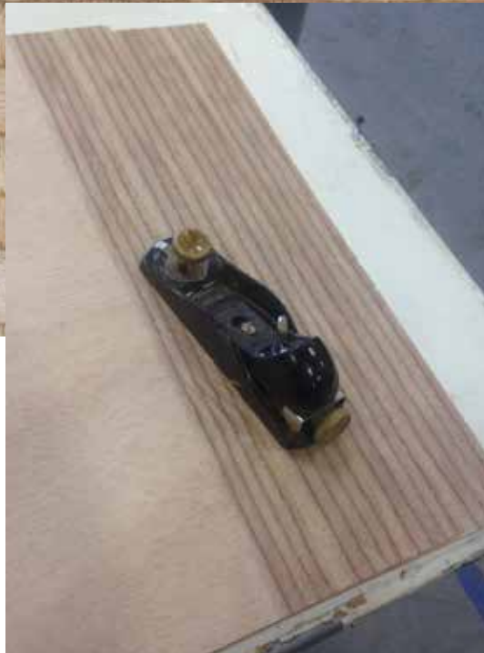
Multiple layers of plywood can be stacked and planed together.
