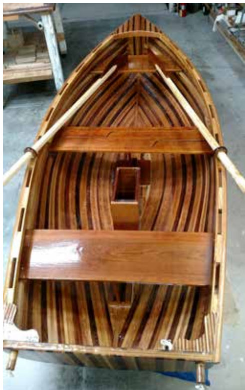
Bill Goddard and Keti Gibbons live in Naples, FL. They built this 9' 10" cedar-strip skiff from scratch using clear red cedar and epoxy.
