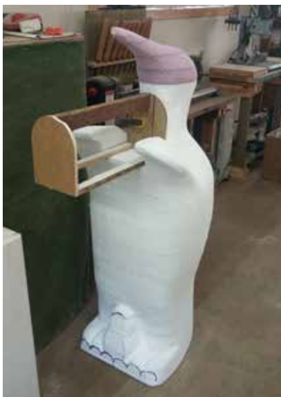
Dry fitting the mailbox form into the shaped Styrofoam mold.
