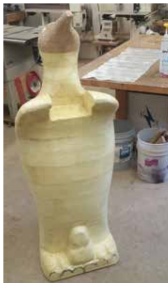
The Styrofoam mold wrapped in fiberglass and epoxy.
