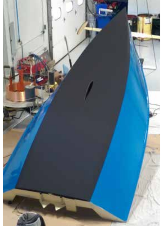
With the hull painted, it was time to roll the boat over and paint the rest of the boat.
