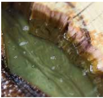
Bubbles rise to the surface of epoxy following a pour. Using a propane torch you can break the epoxy's surface tension, removing air bubbles. Using the multiple pour technique, the result is a 3½" deep casting of 105/207, free of bubbles.
