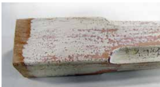
A spindle after two coats of 105/206, one coat of primer and sanded.
