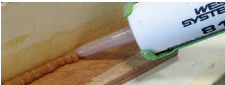
The 810 Fillable Caulk tube allows you to lay down a consistent bead of epoxy.
