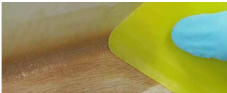
Jack's fast filleting tool is perfect for creating fillets in one pass.
