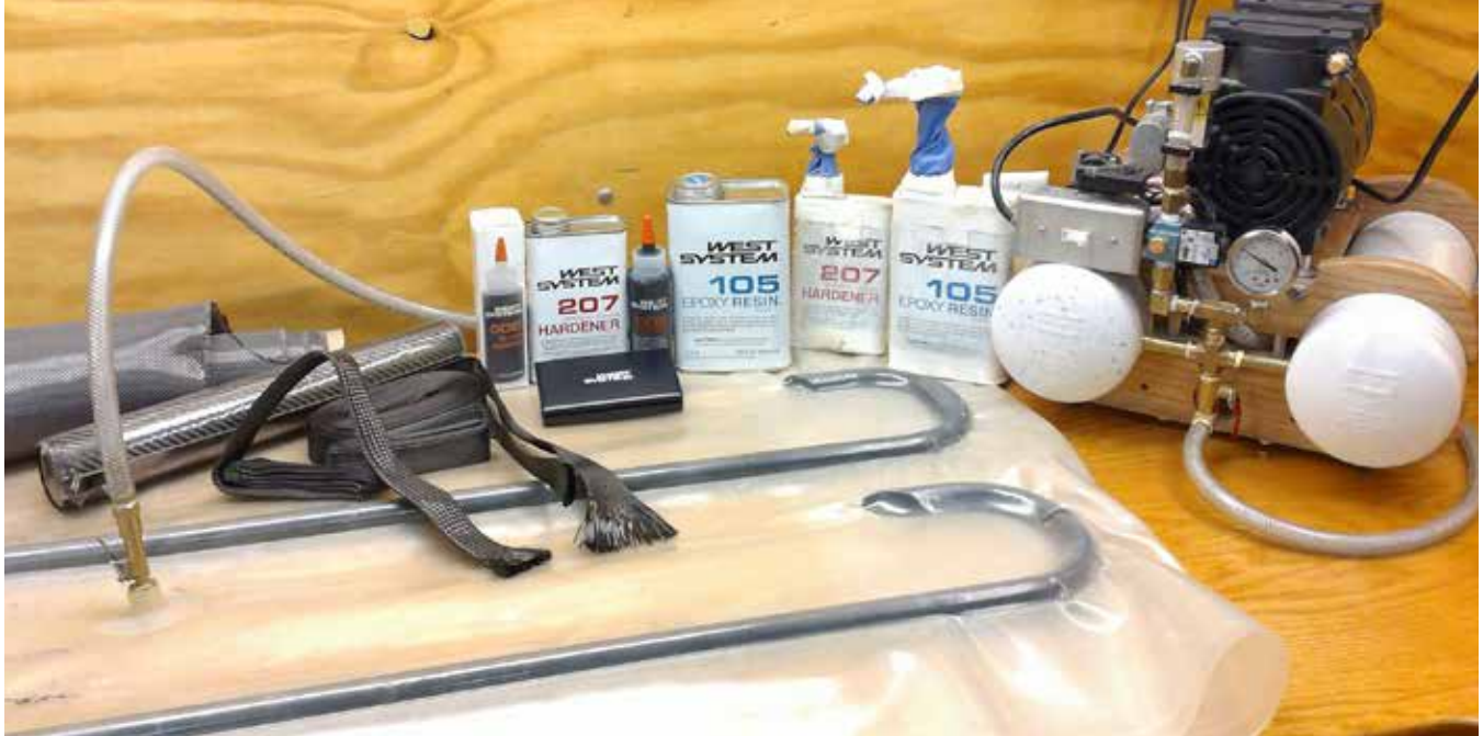
Vacuum bagging setup
