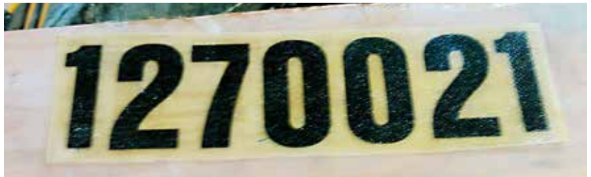
Using G/flex 650 helped Ed avoid much of the mess of mounting documentation numbers onto the bilge.
