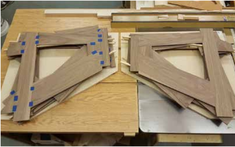
Each half of the main triangle bicycle frame is made up of four layers of 5mm black walnut.
