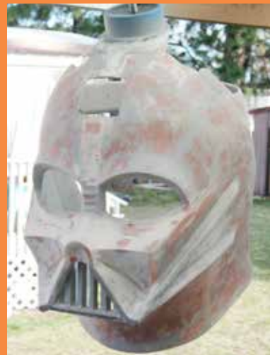
Bottom Right: The fiberglass shell after 105/206 and 407 filler has been applied and faired.
