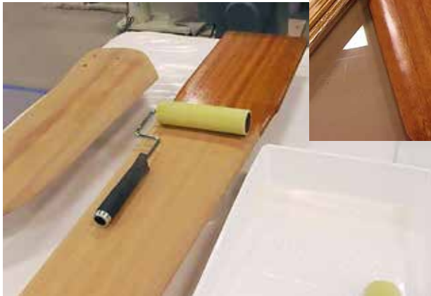
Rudder and dagger board sanded and the first coat of epoxy being applied.
