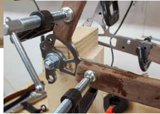
The dropouts bonded to stays. Bolts will be used to secure the dropouts in addition to the epoxy.
