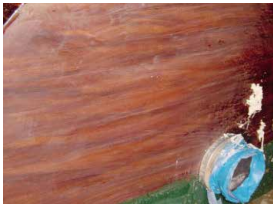
The third pass and ready for sanding. No hints of the major surface imperfections are left. The surface has a nice fine finish, ready for 150-220 grit sandpaper.
