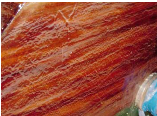
The first pass of scraping. Note the triangular sag in the upper left corner. My roll and tip technique still leaves something to be desired at times. The other ripples and general stippled surface show readily under the first scraping pass.
