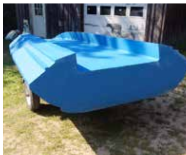
The hull repaired, and faired with WEST SYSTEM Epoxy thickened with high-density and low-density fillers, then gelcoated in blue. We had no problems using the poly based gel coat over epoxy, as we took no shortcuts. Everything was sanded and properly cleaned before spraying.
