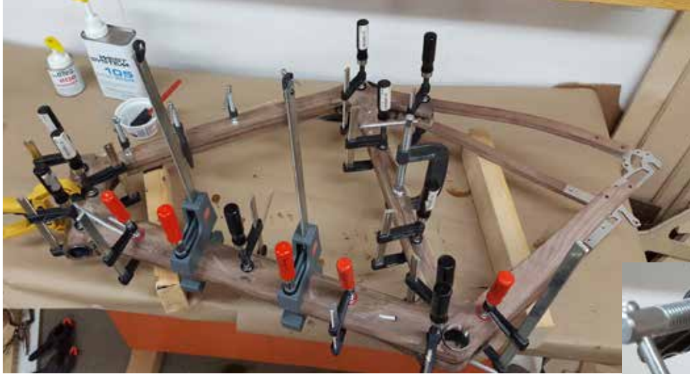
The two halves of the frame becoming one.
