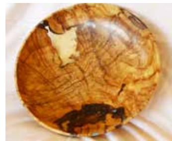
When using 105/207 you end up with clear windows through the side of the bowl.
