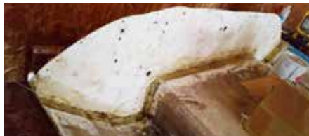
The hull completely gutted of the original deck and transom wood structure
