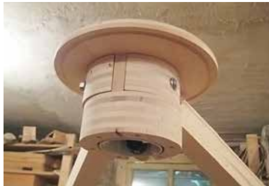
The fan hub assembled with the rooflet ready for epoxy coating and painting.
