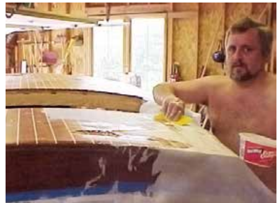
Mark applying fiberglass to the deck. It was 90°F when this picture was taken, but when using epoxy, gloves and a T-shirt are still strongly recommended.
