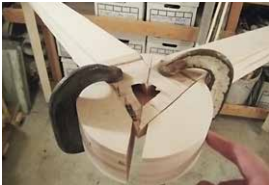
The fan hub clamped to the legs.
