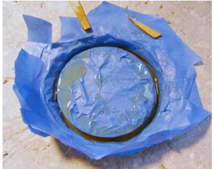
The G/flex 650 collar poured and curing.
