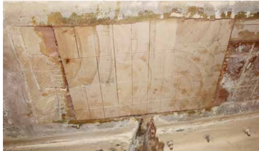
New balsa core epoxied into place where the rotted material had been removed.
