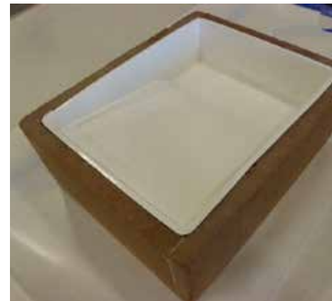
Foam box holding water and a roller pan to help cool epoxy and increase working time.
