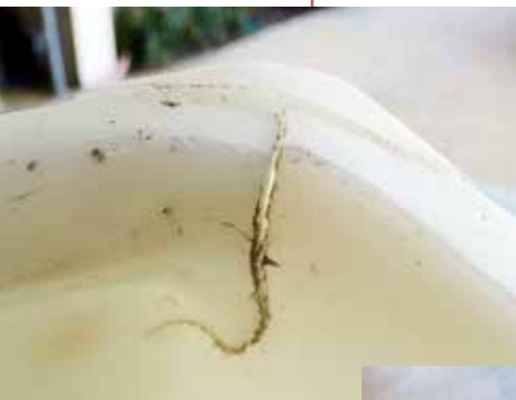
Severe cracking had compromised the structural integrity of the seat.
