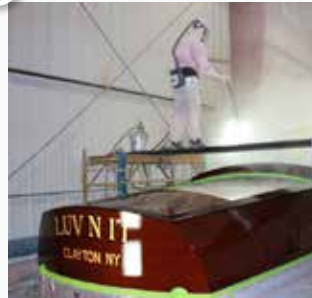
Van Dam is comfortable with multiple finish approaches and finish products. In this case, as on many of its new boats, Trevor Brazell sprays an automotive clear coat over the top of the WEST SYSTEM 105/207 on the exterior.
