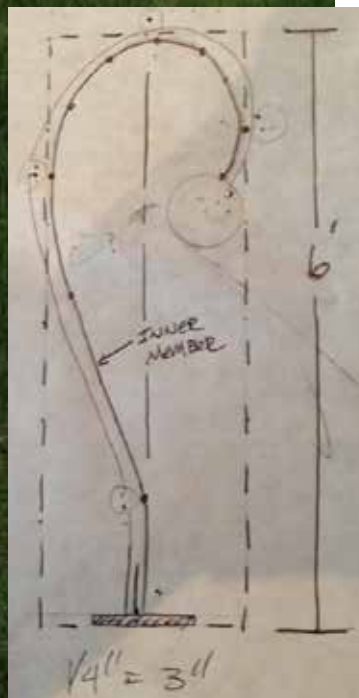
Graph paper sketch. Note centerline of balance and push-pin holes for fairing the curve.
