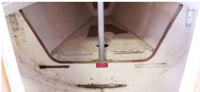
The bulkhead we were replacing, looking from the companionway towards the bow.
