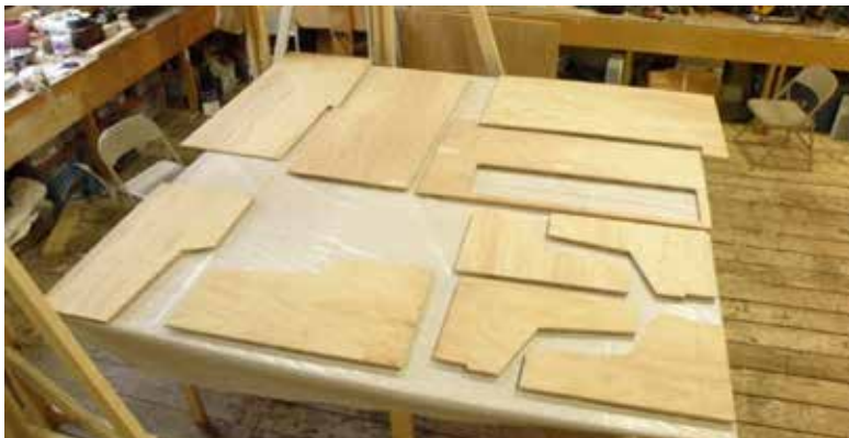
Starting with the many smaller pieces, learning how to measure three times and cut once, then onto epoxy coating and fiberglassing sessions.
