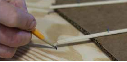
Tom transfers the template points to the plywood.
