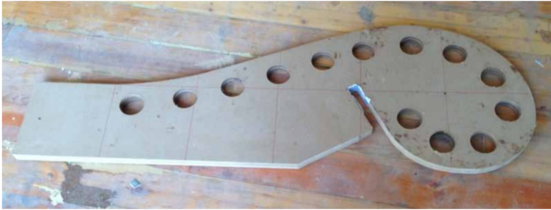
The clamping jig made from laminated MDF. Note the subtle red grid lines scaled up from the design sketch.
