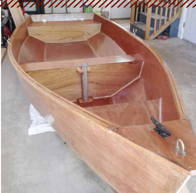
The boat after the epoxy coating was rolled on.
