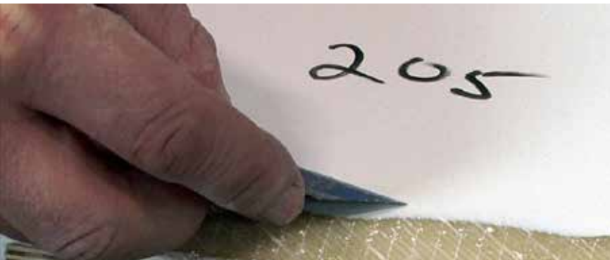
Fine edge bonding test. Scraping the edge of the gelcoat with a razor tests how well the fine edge of the gelcoat stays attached to the epoxy layer below.
