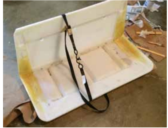
The corners of the seat shell were reinforced with fiberglass tape.
