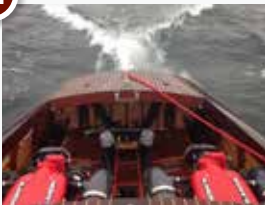
Van Dam does its first of multiple sea trials with engine hatches off and all mechanical and electrical systems accessible. This allows for ready monitoring of all components, assuring a trouble free experience for the customer.
