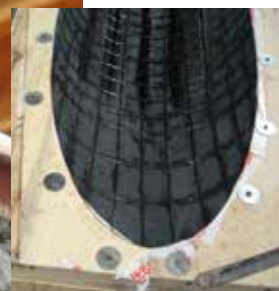
Left, the temporary plywood backer for the flange screwed onto the jig.
