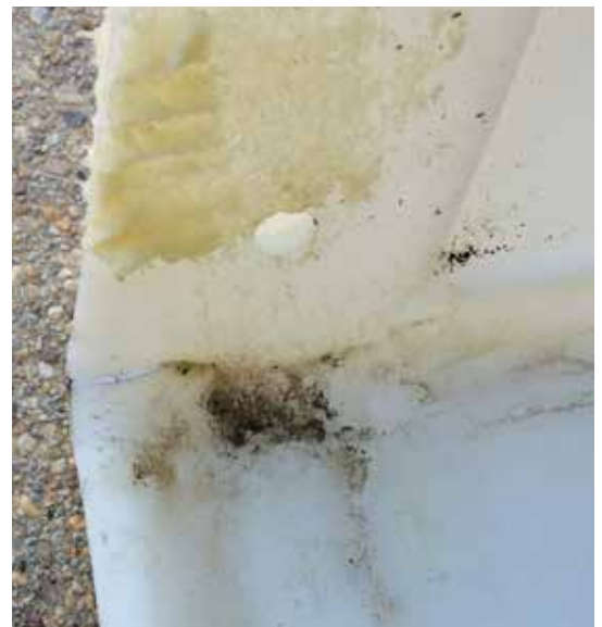
The seat has 18 years of accumulated dirt and residual foam and glue that needed to be removed.
