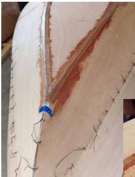
The panels have been stitched and some seams fiberglassed
