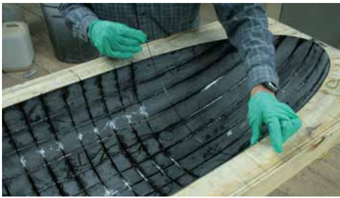
Installing carbon fiber tows inside the dirigible
