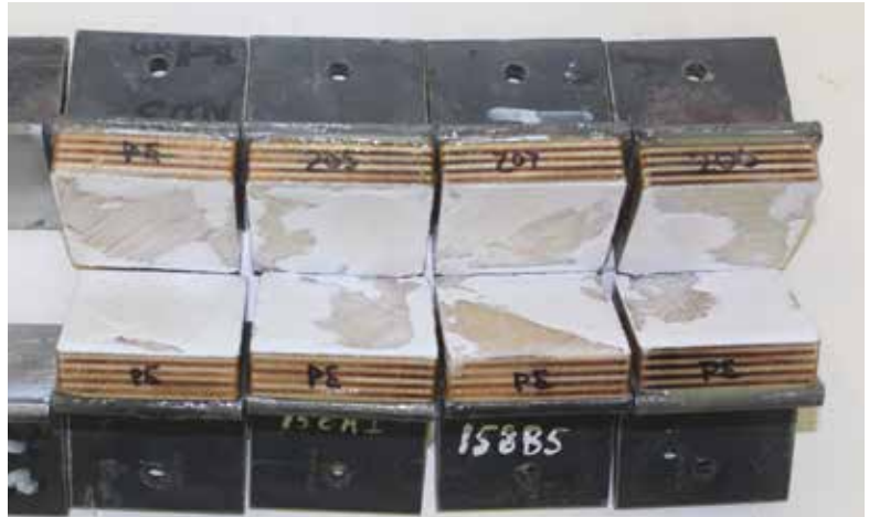
The samples after failure. The results of the maximum loads are listed in the table below.
