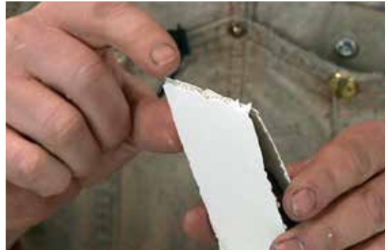
Flex stress test. The panel was intentionally broken in half looking for bond failure along the fracture point.
