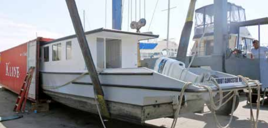
Testing the fit of the completed shipping container boat for low-key insertion and extraction into a standard ISO 40' shipping-container
