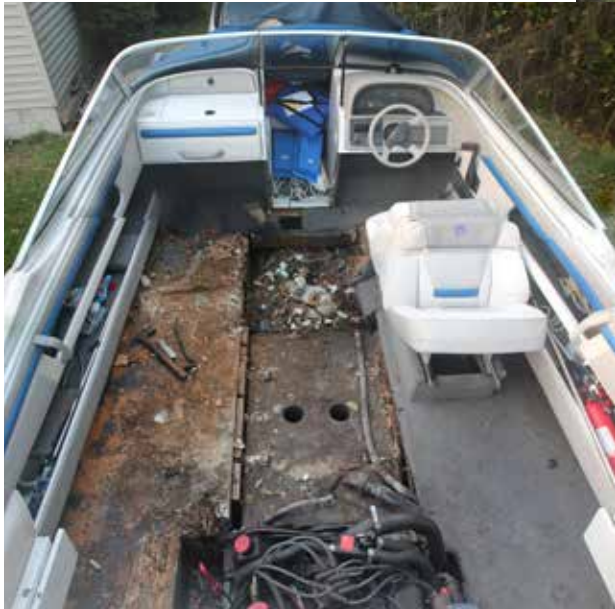
Rotted and damaged wooden cockpit sole
