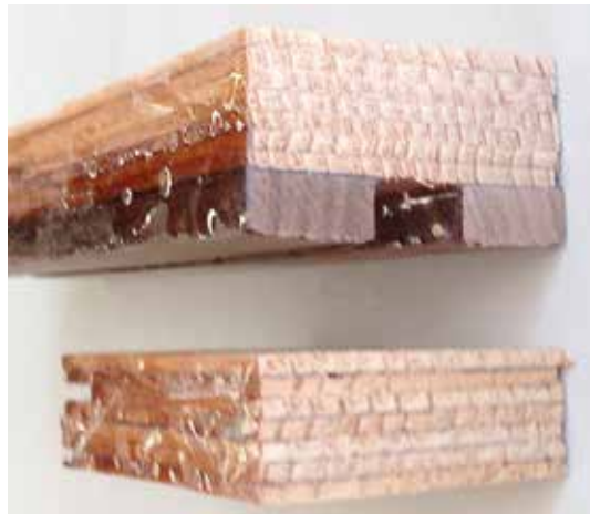
Cut-offs of the laminations showing the inside and middle member lamination ready for lamp cord and then outside lamination.
