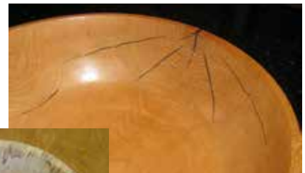
Turned pieces that had cracks filled with graphite powder creating the same effect as using 502 pigmented epoxy
