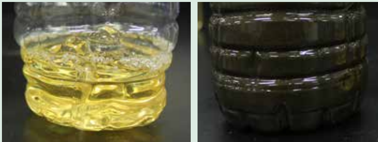
Left: A 1 inch deep pour (70 grams) of 105/206 in an 18 oz. bottle reached 410°F, cracked and deformed the bottle.
