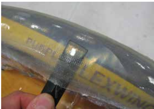
A mixing stick is used to start to pry the cured epoxy and fiberglass away from the mold.
