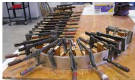
Top: A polyethylene sheet is used as a mold release for the foam core bracket Bottom: The bracket laid up and clamped
