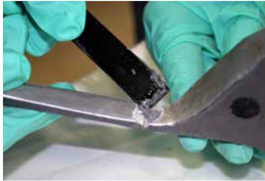
Left: Prepping the surface by sanding with 80-grit sandpaper. The metal support rod was exposed when the plastic broke.
