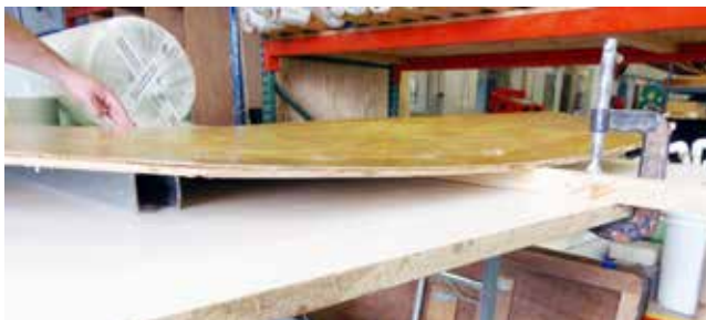
Applying a 1" rocker to the mold surface
