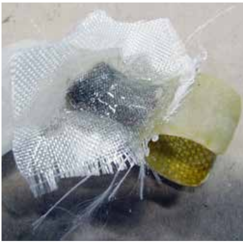
Left: Fiberglass wrapped around the foam spacer
