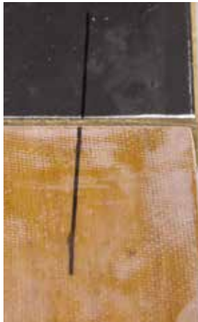
Left: All sides liberally coated with WEST SYSTEM 105/207 with 410 Microlight filler to create a smooth finish.
