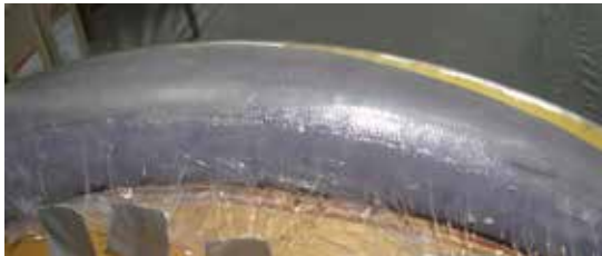
Fiberglass applied to the mold surface.
