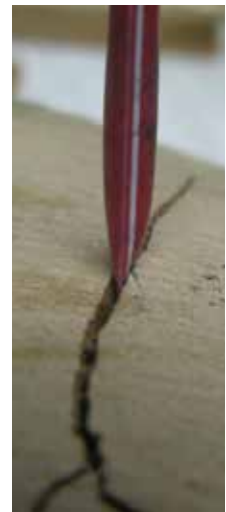
Bottom Right: Close up showing how the plastic straw extending the syringe tip conforms to narrow cracks
