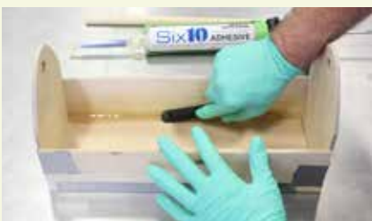
Fillet being applied to joints
