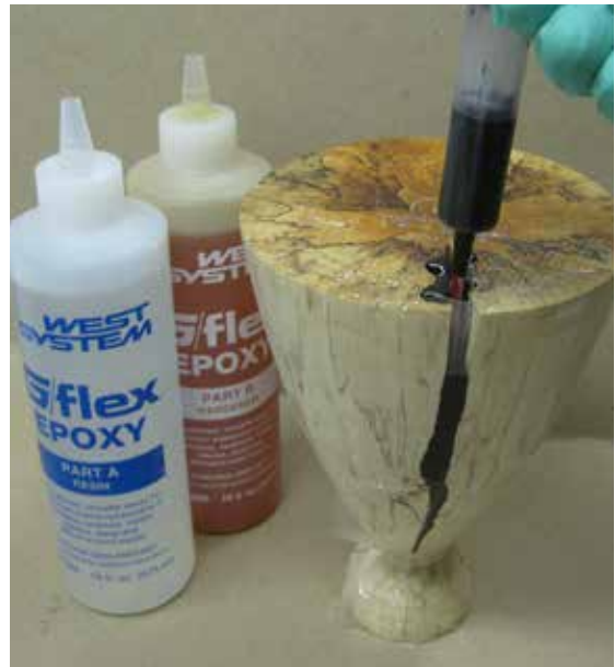
Bottom Right: Close up showing how the plastic straw extending the syringe tip conforms to narrow cracks
