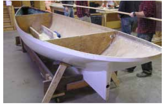
Top Right: The school accepted this 20' fiberglass launch as a commissioned job to modify and finish the interior structure necessary to convert it into an electric launch and to install a wood/composite deck.
