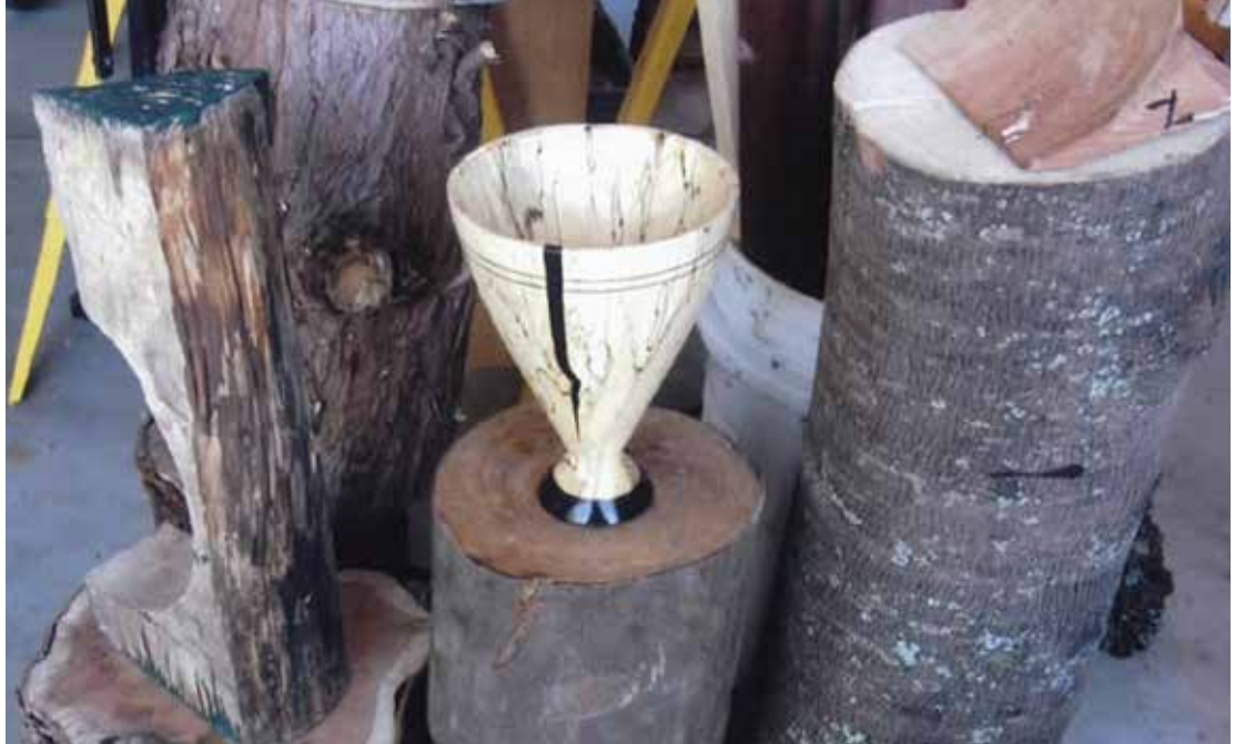
Turned wooden goblet. The cracks are filled with G/flex 650 and black pigment.
