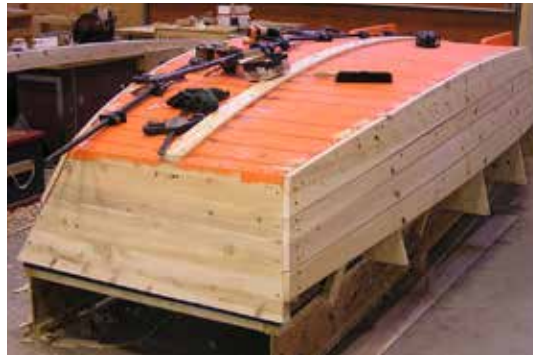
Bottom Right: A Garvey work boat—a 16' design that utilized the scantlings from the original 19' 7" design built at the Mystic Seaport Museum. It will be driven by an outboard engine mounted in an inboard well and, like the original, it will help move GLBBS boats. This build is a replica of a 100-year-old design sold by the Petoskey Boat Co.
