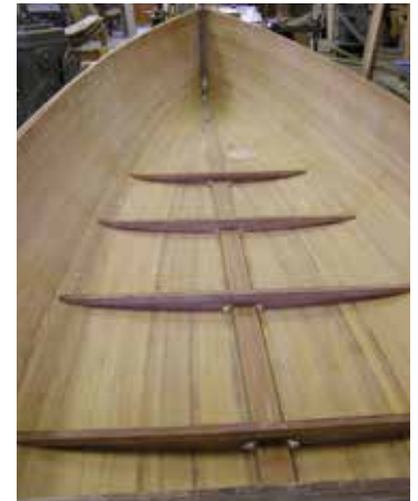
Bottom Right: This is a cold molded, cedar strip and glass, vacuum bagged hull that was built at the school and had been sitting for a couple years and not getting much attention—so Andy bought it for himself. He's in the process of adding floors and interior structure. Eventually, it will have a cuddy cabin and be powered by a 15–25 hp outboard engine. Perfect for toolin' around Les Cheneaux.
