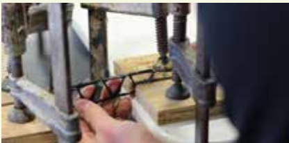
Bridge being placed between vertical supports for testing
