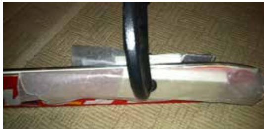
Clamped and curing at 68°F
