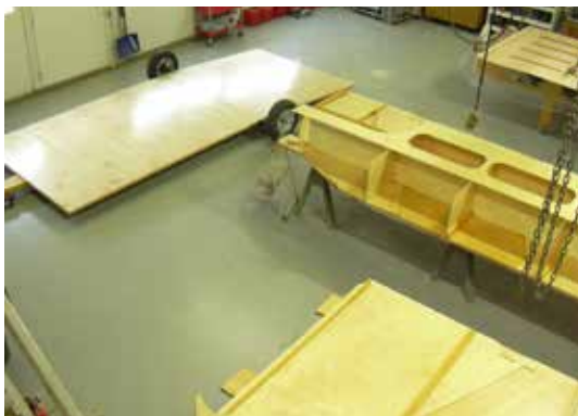
½" Baltic Birch Plywood was used for the trailer floor.
