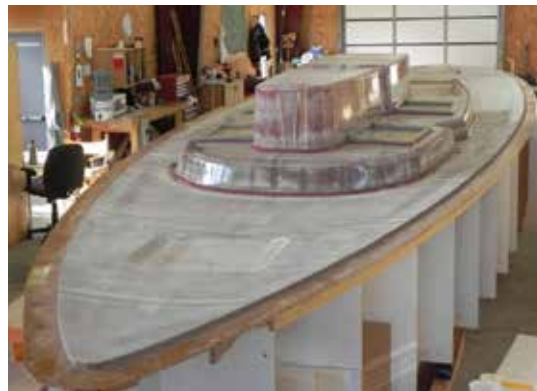
The deck was constructed with fiberglass skins and foam core vacuum bagged with WEST SYSTEM 105 Resin and 206 Slow Hardener.
