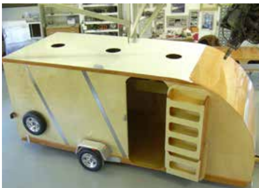
Storage compartments were built into the door for tools needed at the race track.
