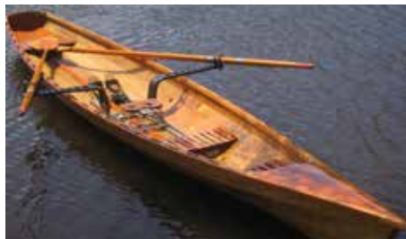
Rob Caveney built a 18' 9" Whitehall pulling boat named Indian using WEST SYSTEM Epoxy.
