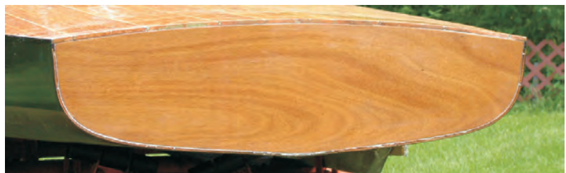
The new transom glued in place, ready for new gudgeons and a new aluminum rudder.
