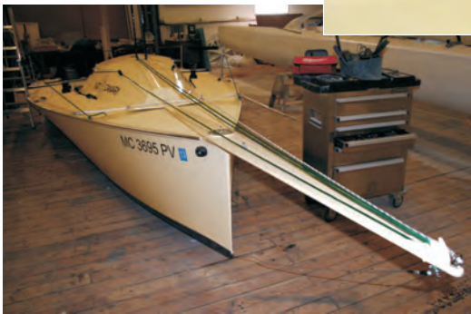
Left —The bowsprit is hinged at the bow and attached to a crossed line at the base of the cockpit (above) which will allow it to pivot 30°.
