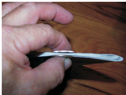
Thickness dictates laminate stiffness. Matching laminate thickness will generally result in similar stiffness to the part you are replicating.
