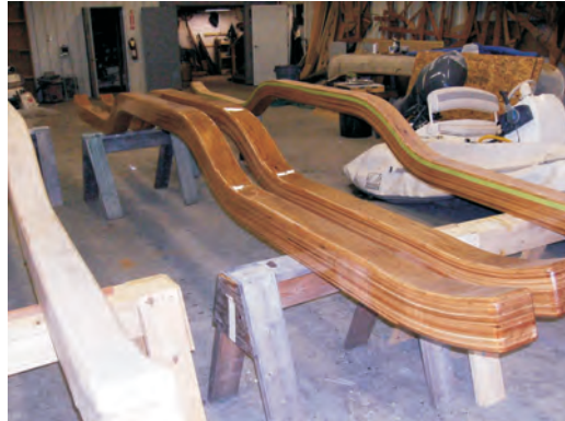
Left —A laminated iako is being planed to final thickness.
