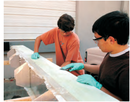
Right—Kell students prepare a laminated hull for fiberglassing (above) while other students begin to trim the excess fiberglass from a hull after the epoxy has cured (below).
