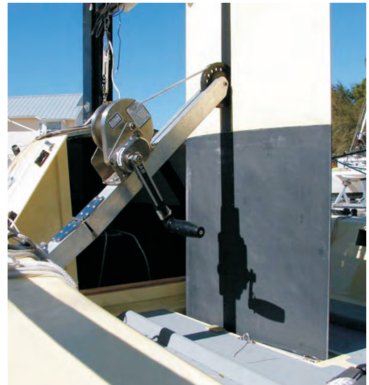
Right —The aluminum crane fits into a slot on either side of the hull and can lift the keel for sailing in shallow water or trailering.
