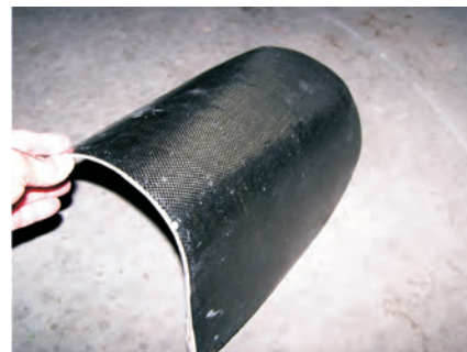
The part with woven carbon fiber bonded to each side.
