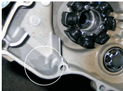
▼ The repaired cover showing the repair area from the inside.
