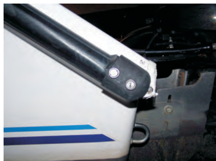
The finished rail cap installed.
