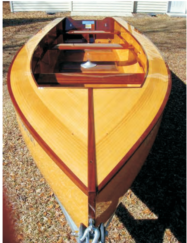
Matthew Gunning of Gunning Wooden Boats LLC, Summerville, South Carolina, sent this photo of a 15' strip boat he built for a customer in Virginia. He used 105 Resin/207 Special Clear Hardener™ with 7.5oz fiberglass cloth on the exterior and 6 oz cloth on the interior.
