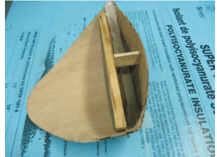
Two plywood panels are joined over a temporary form to produce the desired shape.
