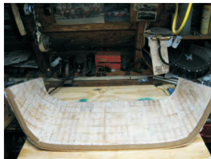
The bench top provides a flat surface while the gussets (hidden in this photo) establish the curvature.
