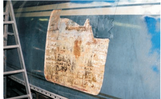
The boat is upside down and the outer skin and core have been removed with a router.
