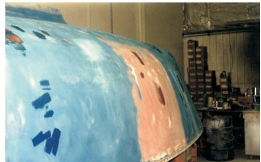
With new skin and core in place the repaired hull was faired before barrier coating and painting.
