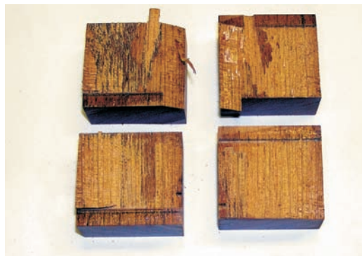
Close up of broken jatoba short block shear test samples. The denser jatoba also failed in the wood grain rather than the glue line.
