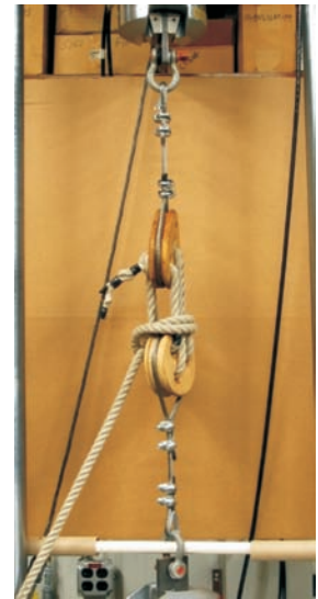
Figure 2, left—The test assembly before testing. The “experimental” two-piece deadeye is on top.
