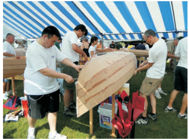
On day two the bottoms of the interiors were fibreglassed. The now rigid hulls were rolled over and the copper stitching was removed.
