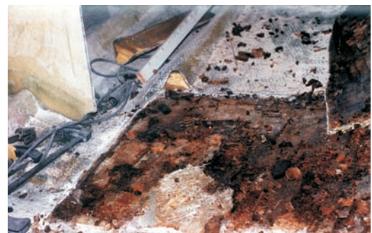
The interior floor skin and rotted balsa core were removed.
