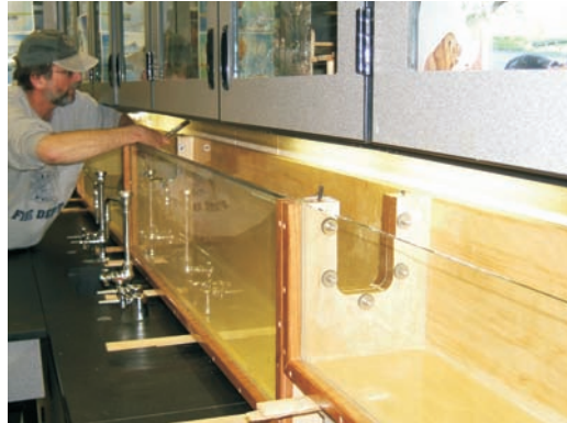
Filipiak assembling and leveling the finished tanks. The tempered glass face was sealed in place with aquarium silicone seated in a groove around the facing of the tank and held in with epoxy coated hardwood retainers.
