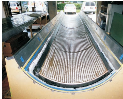
The cured outer carbon skin with foam core.
