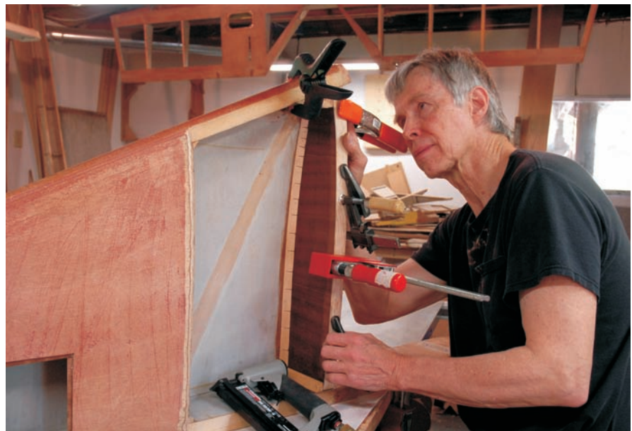
After checking the rib's alignment, the author clamps and staples it in place before the epoxy sets.
