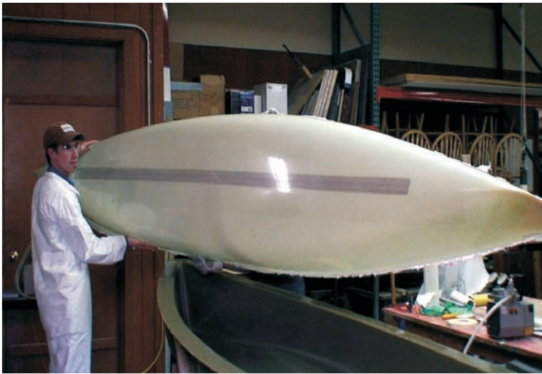
Chad Sinicki removes his third hull from the mold. The hull, three layers of 737 Biaxial Fabric was the first one he vacuum bagged.
