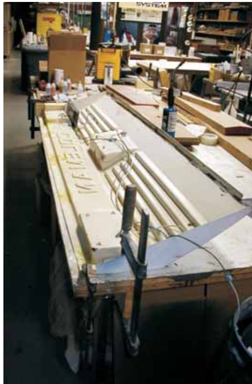
The grill is clamped to remove twist while the repairs are made and the epoxy cures.
