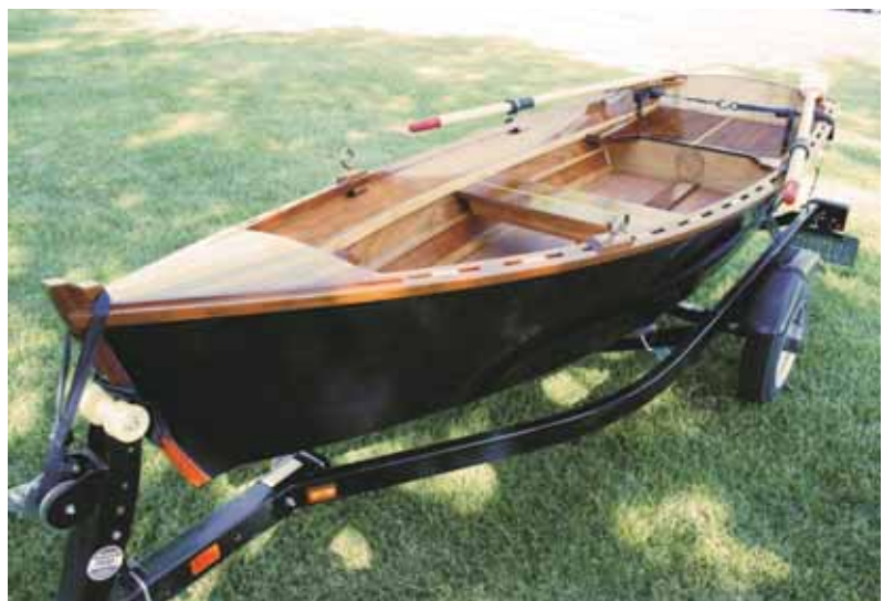
The interior was left natural wood—seats, bow deck and gunwales are mahogany with Sitka accents. The hull is painted with House of Color™ Midnight Blue Pearl.
