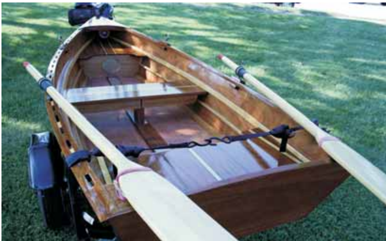
Three more views of the completed Sand Dollar. The varnished interior has 10 to 12 coats of Captain's Spar Varnish™ over the 105/207 epoxy-coated surfaces.
