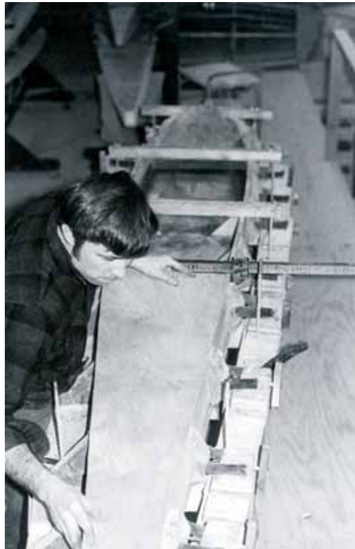
Joel Gougeon fits a plywood deck to the hull of one of the more than 200 DN iceboats built by Gougeon Brothers.
