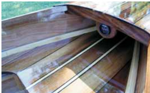
Three more views of the completed Sand Dollar. The varnished interior has 10 to 12 coats of Captain's Spar Varnish™ over the 105/207 epoxy-coated surfaces.
