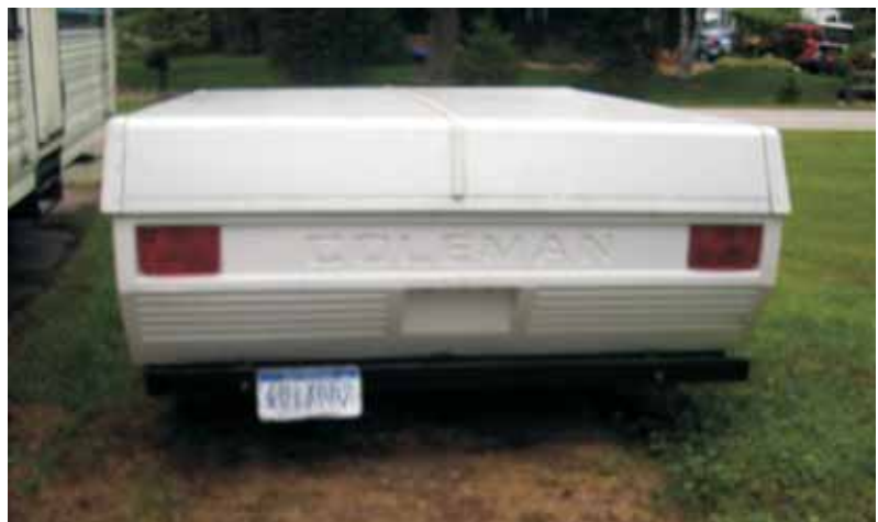
The repaired panel is back in place on the camper. A coat of Krylon Fusion™ textured, plastic-compatible paint completed the repair.
