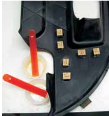
1—Test blocks glued to the underside of the cover.
