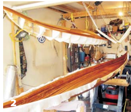
1—The stripping of the hull with western red cedar is completed.
