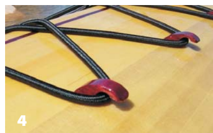
3 & 4—Purpleheart provides a nice contrast for the outline of the deck design and deck hardware. Everything is coated with 105/207 and finished with 5 coats of Z-Spar Captains Varnish.
