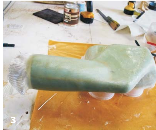
3—The fiberglass has cured over the Styrofoam mold before it is trimmed and sanded.
