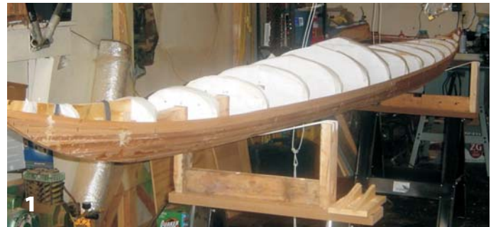
1—The stripping of the hull with western red cedar is completed.
