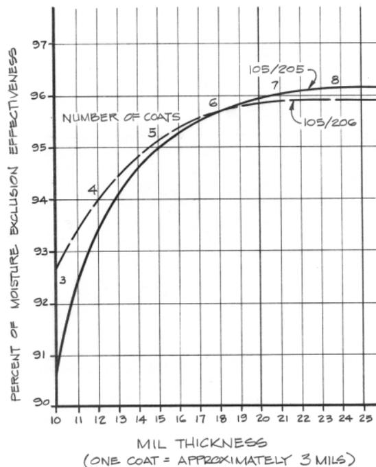
Figure 2—Effect of film thickness on MEE
