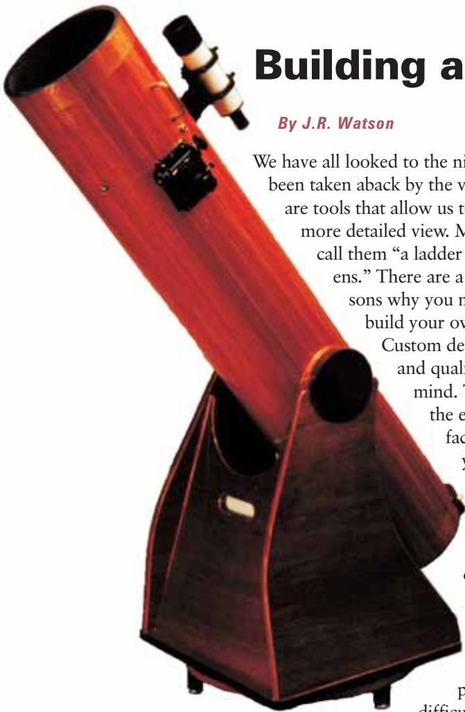
A portable, easy to build, cedar strip reflecting telescope.
